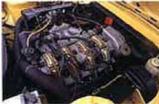
Separate rocker covers were a typical NSU feature and were carried over for the K 70
